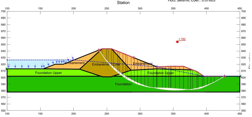
Name: Embankment Unit Weight: 117.5 pcf Cohesion': 1,120 psf Phi 1: 9.5 ° Constant Unit Wt. Above Water Table: 101 pcf Name: Foundation Unit Weight: 115 pcf Cohesion': 315 psf Phi 1: 30.5 ° Constant Unit Wt. Above Water Table: 111 pcf Name: Embankment Core Unit Weight: 109 pcf Cohesion': 1,120 psf Phi 1: 9.5 ° Constant Unit Wt. Above Water Table: 101 pcf Name: Foundation Upper Unit Weight: 118 pcf Cohesion': 365 psf Phi 1: 30.5 ° Constant Unit Wt. Above Water Table: 115 pcf
