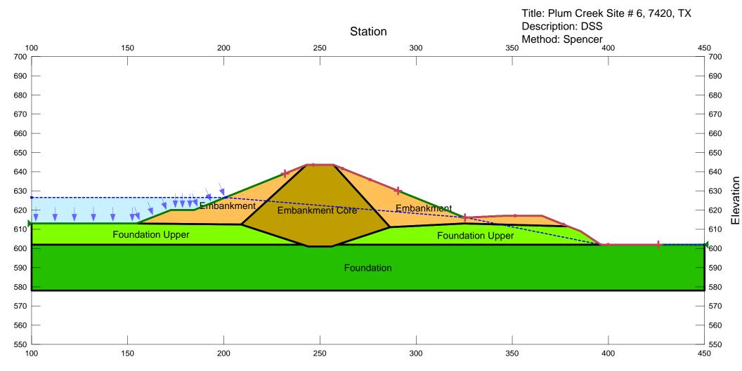
Name: Embankment Unit Weight: 117.5 pcf Cohesion': 1,120 psf Phi 1: 9.5 ° Constant Unit Wt. Above Water Table: 101 pcf Name: Foundation Unit Weight: 115 pcf Cohesion': 315 psf Phi 1: 30.5 ° Constant Unit Wt. Above Water Table: 115 pcf Phi 1: 9.5 ° Name: Embankment Core Unit Weight: 109 pcf Cohesion': 1,120 psf Constant Unit Wt. Above Water Table: 101 pcf Name: Foundation Upper Unit Weight: 118 pcf Cohesion': 365 psf Phi 1: 30.5 ° Constant Unit Wt. Above Water Table: 115 pcf
