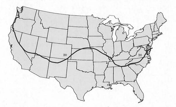
Figure 523-1 Number 20 Freeze-Thaw Severity Index Isoline (map approximates the map in ASTM D5312)
